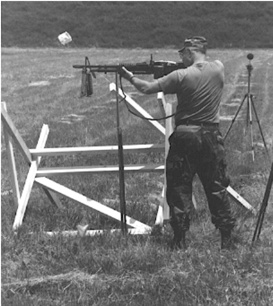
Figure 2. Unmuffled M-60 being fired at the center of the instrumentation circle during close-in noise level measurements.
