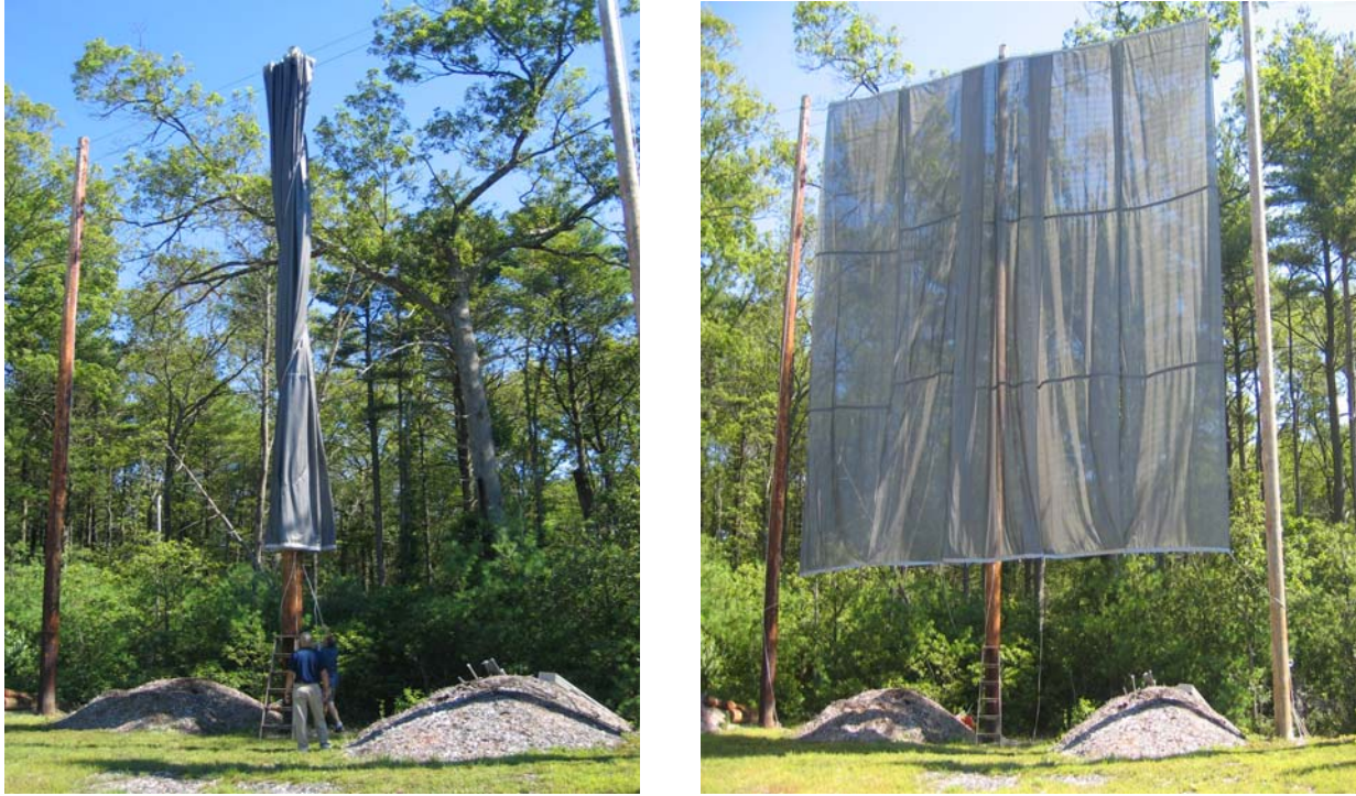
Figure 10: Photograph of Draw-Drape LSC Design Developed by the Standish Sportsmen’s Association; LSC Deployed at SSA, East Bridgewater, MA
